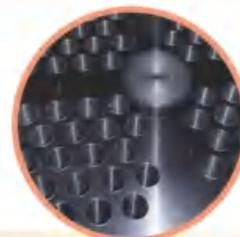
Workpiece: Plates of condenser pipe
