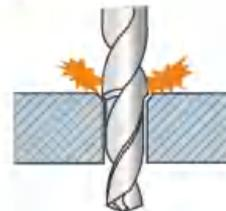
When countersinking, cutting force increases at initial stage. Please reduce the feed.
