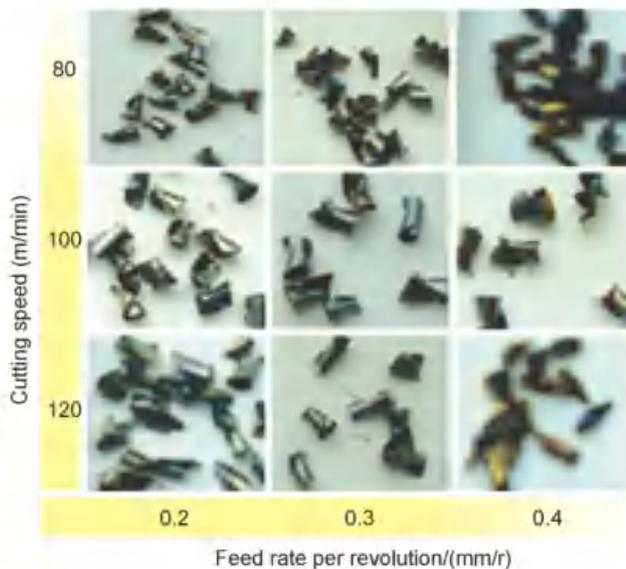
**Good chip breaking capability and stable machining with different cutting speed and feed rate.**
