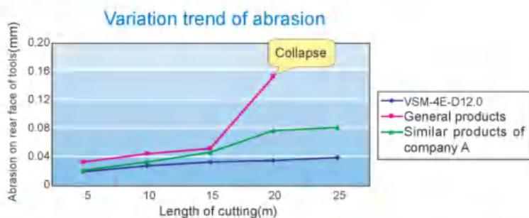
Note: ◆ Compared with competitor's, VSM end mills can perform better on wear resistance and tool life.
