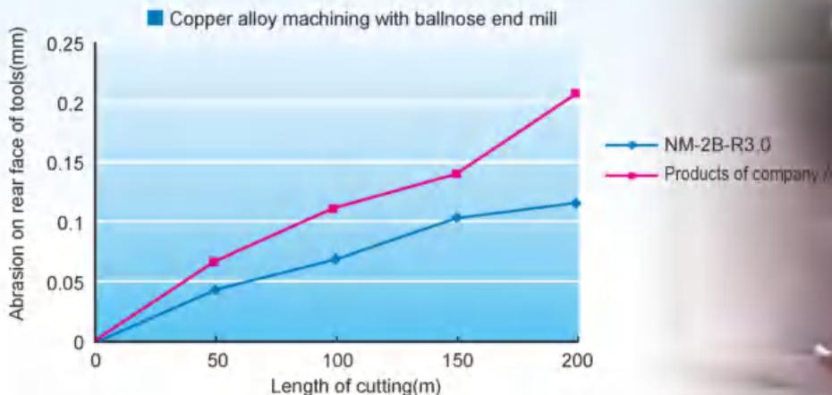
NM series for copper machining
