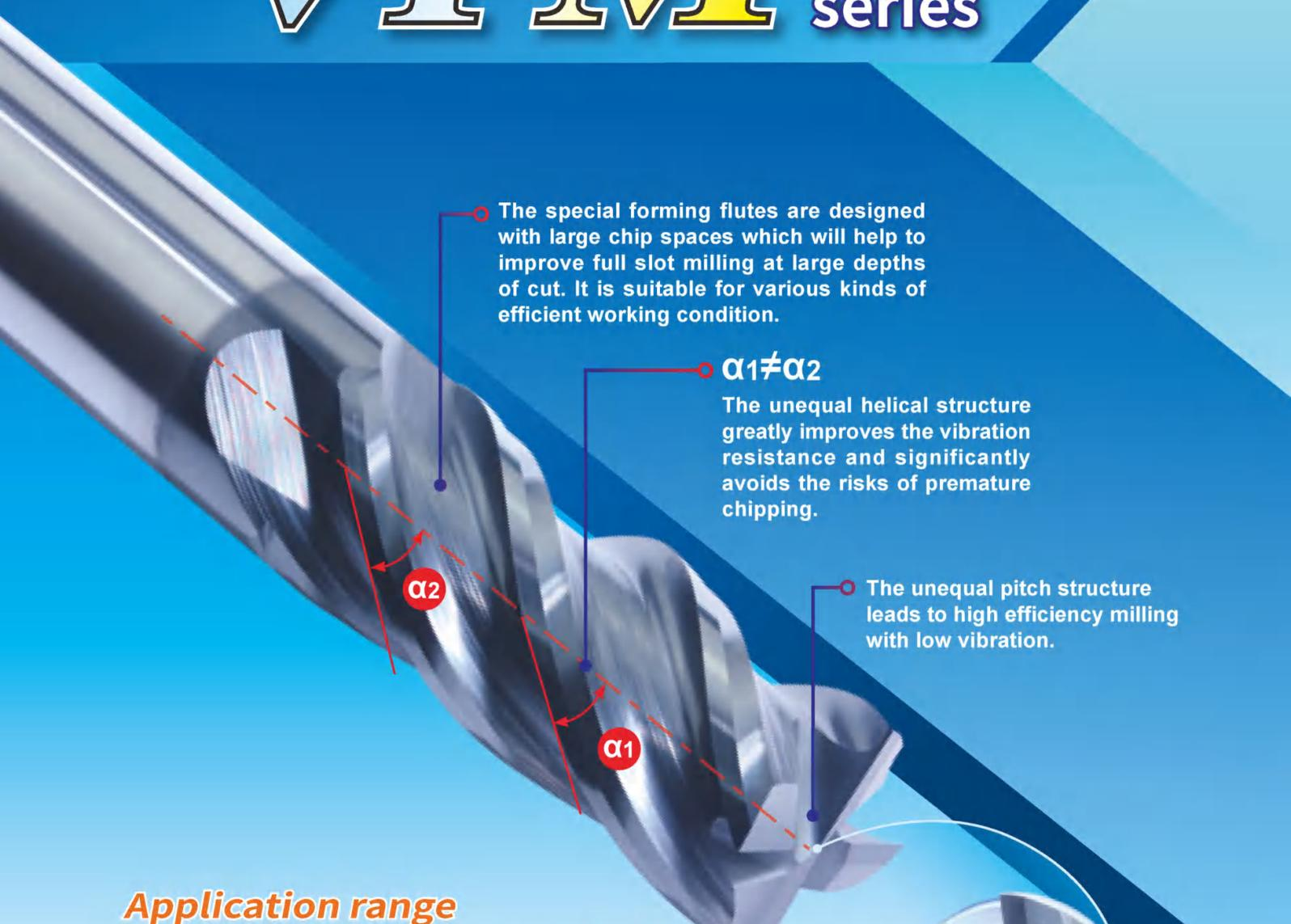
The special forming flutes are designed with large chip spaces which will help to improve full slot milling at large depths of cut. It is suitable for various kinds of efficient working condition.
