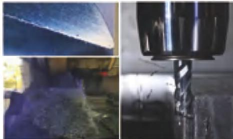
**Test result: After processing 120 meters, the normal flank wear of our cutting tool reaches 0.039mm which can still work.**
