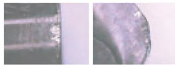
ZCC-CT insert after 80 minutes machining
