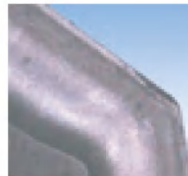
Abrasion on rake face
